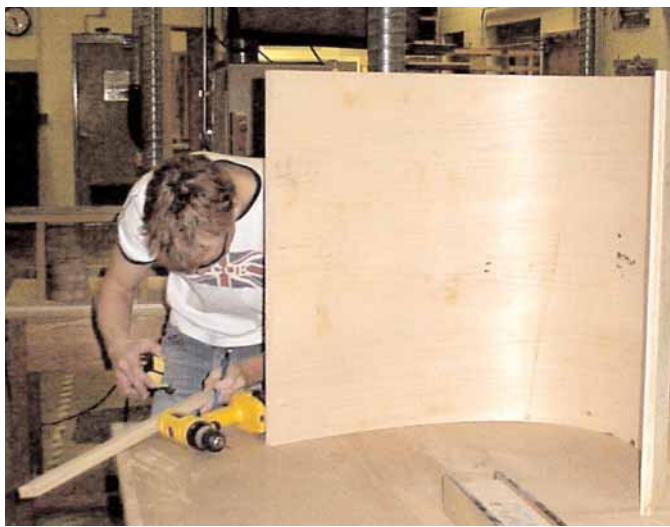
Using measurements from the left-side drawer casework, Emory prepares parts for the jig to hold the piece for the table saw pass that will square off the ends.
