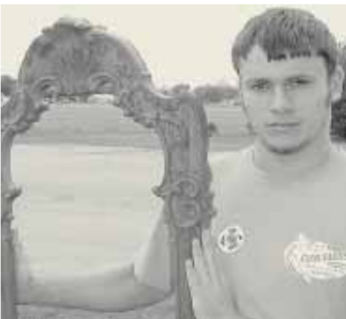
Paul Wilson, whose French provincial table achieved for him first-time-out recognition at AWFS, displays a Rococo mirror frame he Mastercam/Thermwood-routed from four pieces of African vermilion (padouk) cut and fixtured so that the grain is vertical throughout the assembled piece.
