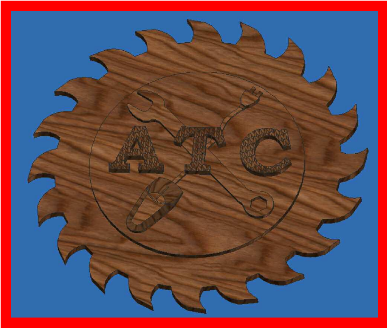
Completed Project. This design used 2D, 2.5D and 3D tool paths created in Mastercam CAD/CAM software and cut from oak on a CNC Lathe to simply depict all of the programs offered at the Advanced Technology Center.
