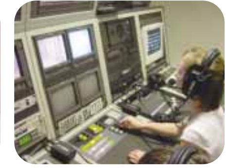
The videoswitcher, Mary Dion, is bringing the proper video source up onto the screen and creating transitions to get from one piece of video to another.
