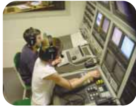
Matt Atwater and Mary Dion work together on the character generator and video switcher to create the video, transitions and word screens necessary to complement each other in a production.
