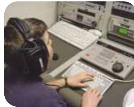
In the control room, Matt Atwater installs the character generator that brings words up onto the program monitor at desired moments of the production.
